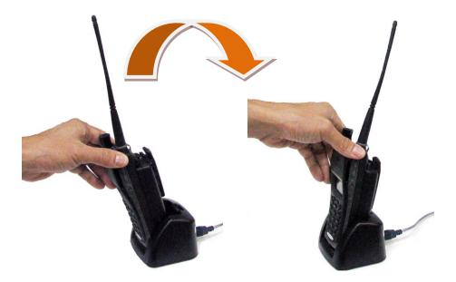
Insert the phone bottom at an angle with its antenna tilted towards you and "rock it back" into place.
